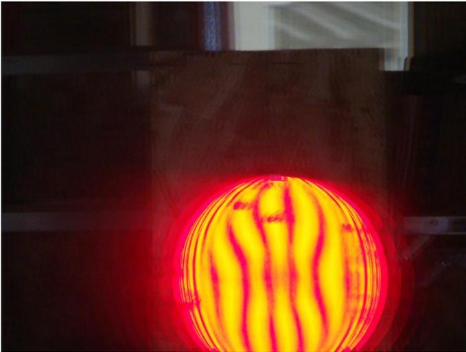
It actually indicates that the center is still high and with the shadow in the center you can tell that it is not polished. We can also see that by looking at the blank but Lee built this tester and we wanted to test it. We will take more images as he finishes polishing and figuring and we will show everyone how it progresses.
